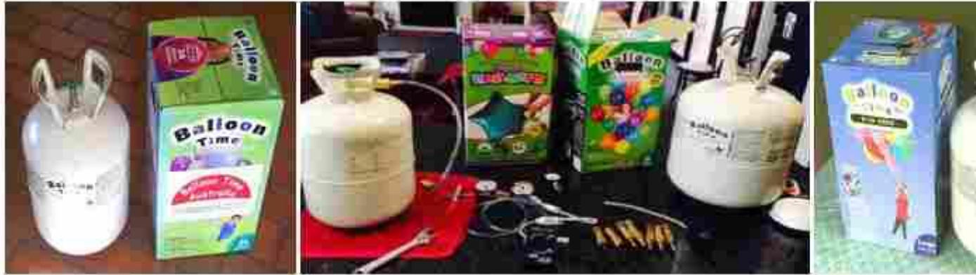
Testing Balloon Time Helium cylinders for Oxygen contamination
