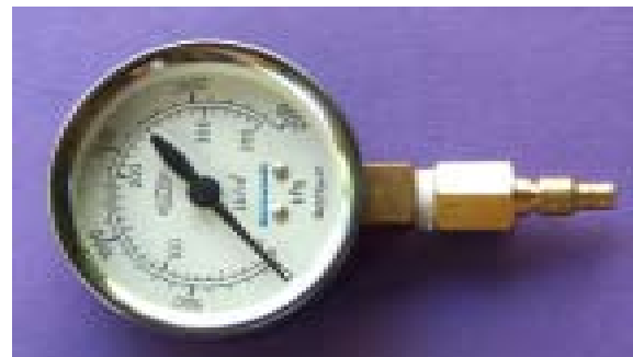
Gauge for tank testing - available on loan from Exit Chapter Leaders
