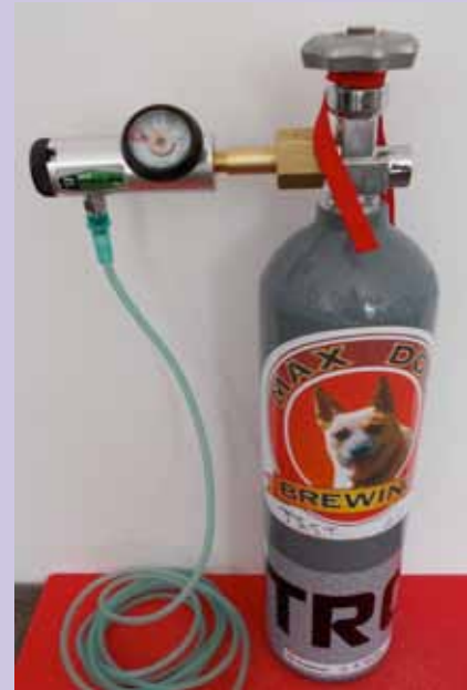
Above: An Australian MDB Nitrogen cylinder
